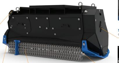
Single Double Chain Curtain Protects Operator from Flying Debris
