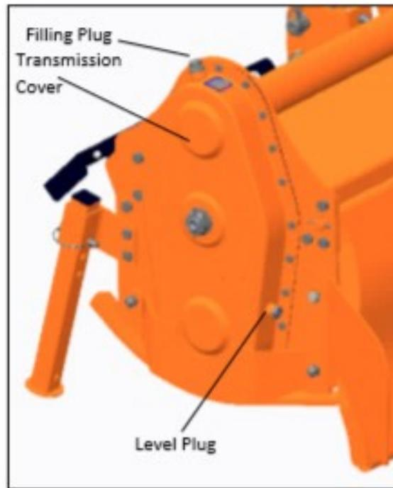
Check the oil level every 50 hours, making sure it reaches the level plug on the transmission cover.
