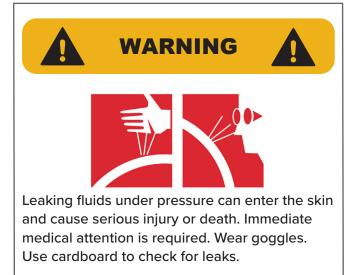
Check condition of all hydraulic components for leaks. Repair as required.
