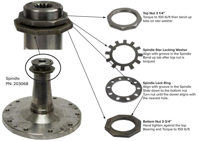
Use red Loctite on the threads of both the lower and upper nut.
