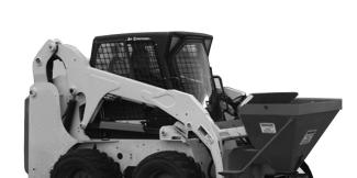
Raise the material spreader to a minimum of 20 in. (508 mm) off the ground and adjust the material spreader level to the ground [Figure 14].
