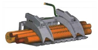
back and retighten the clamp arm pressure. When rolling back the attachment, the load will settle and require some additional clamping pressure to secure the load.
