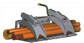
7. After loading your attachment and clamping the arms over the load, roll the attachment back and retighten the clamp arm pressure.
