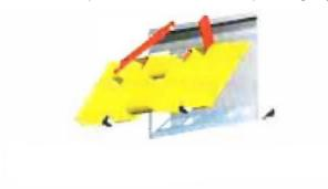
When the top edge of the coupler is seated in the top part of the coupler plate, roll the skid steer tilt function back until the attaching plate is flat against the skid steer coupler. Lock down the coupler levers.
