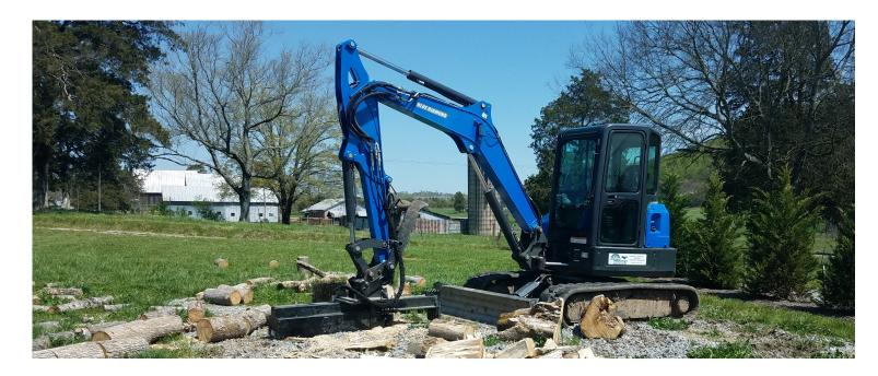
The Blue Diamond® Heavy Duty Excavator Log Splitter is a great tool to get your firewood ready. Fit up to 22" logs and split them with the powerful 25-ton cylinder. The bolt-on mounting plate allows the operator to switch mounts when changing machines. It can be mounted parallel or perpendicular to the operator for visibility preference. The reinforced tubular frame is designed to withstand many years of use.
