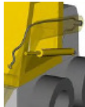
Route harness to back of loader pivot and on the inside of loader arm
