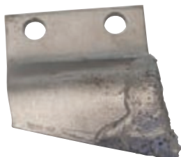
Left Cup Tooth (48" trencher) 231018
