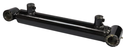
Cylinder 2" Bore, 10" Stroke (1/4" ports, fits SD Grapple Bucket) 206306
